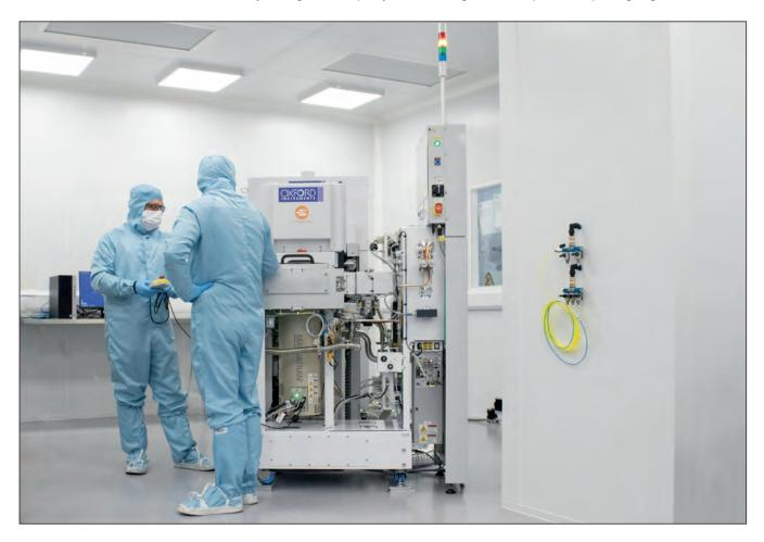
For many years, Plasma Technology has offered tools for inductively coupled etching. Very recently, they have been complemented with equipment that can remove material by one atomic layer at a time. Together, these two etching techniques are ideal for the production of normally off AlGaN HEMTs, which have very thin layers, and a two-dimensional electron gas that must not be damaged
