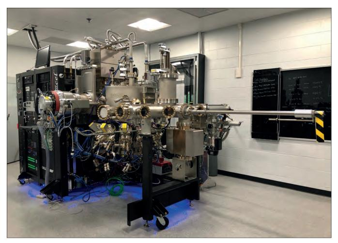
Veeco GenXcel oxide MBE tool located at AFRL dedicated to fundamental oxide materials and device research on up to 4-inch substrate sizes.
